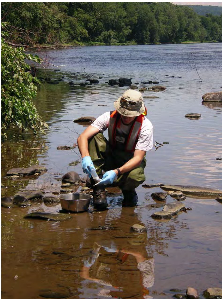
John Clune, PA Water Science Center, Collecting an emerging-contaminants bed-sediment sample at the Susquehanna River at Danville, PA. (Photo by Collie Loper, USGS)
