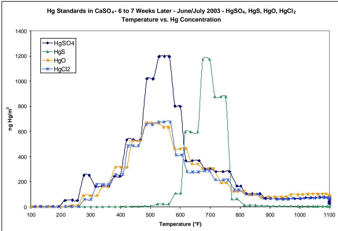
Figure 6: Thermodecomposition Profiles of Site-Collected FGD gypsum
