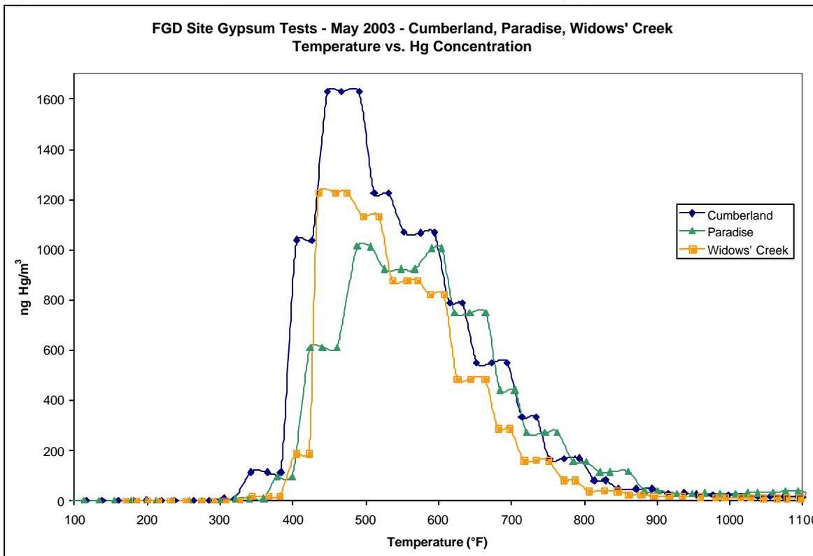
concerned the temperature at which mercury began to evolve, 200°F for the mercury-amended samples compared to 390°F for the site-collected FGD samples. The Cumberland sample evolved mercury at 340°F however the sharp rise began at 390°F
