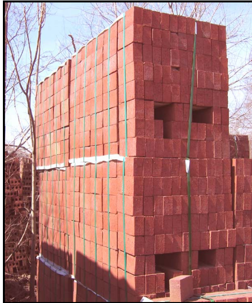
Figure 7: Run II: 2000 paving bricks containing 20 vol% CPSIC fly ash
