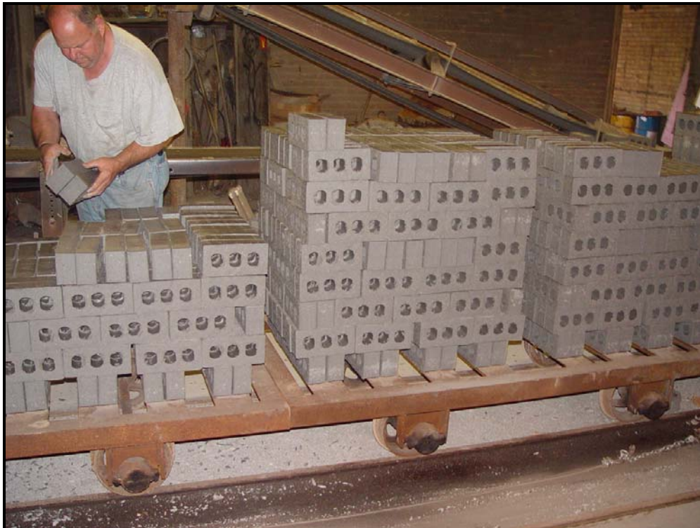
Figure 8: Scale-up extrusion at the brick plant produced three-hole green building bricks (700 bricks per car)
