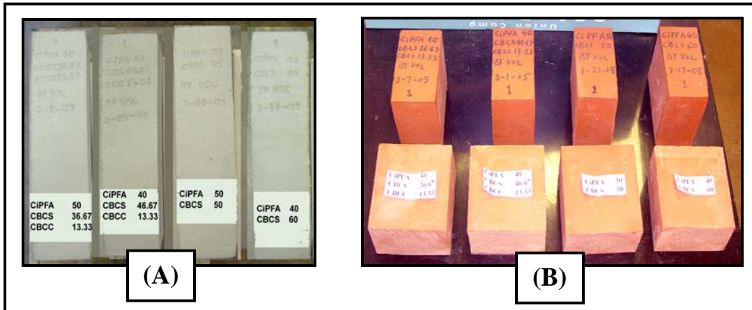
Figure 6: Mold-pressed paving bricks containing 40 and 50 vol% fly ash, balanced with shale and clay, before firing (A) and after firing and then splitting in half (B)
