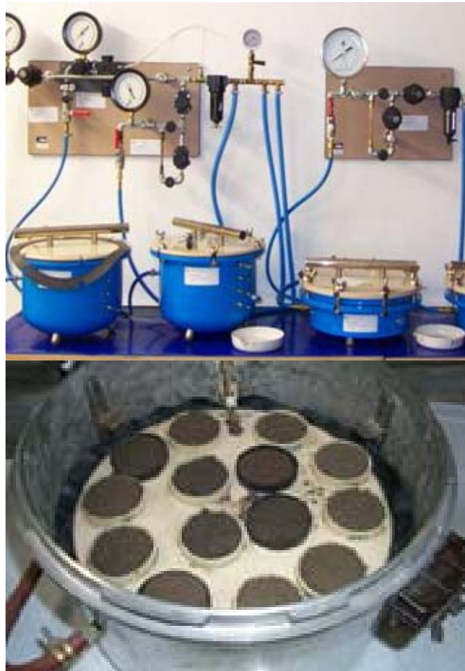
Figure 7. Schematic of packed soil column (top), and pressure plate apparatus (middle) and (bottom).
