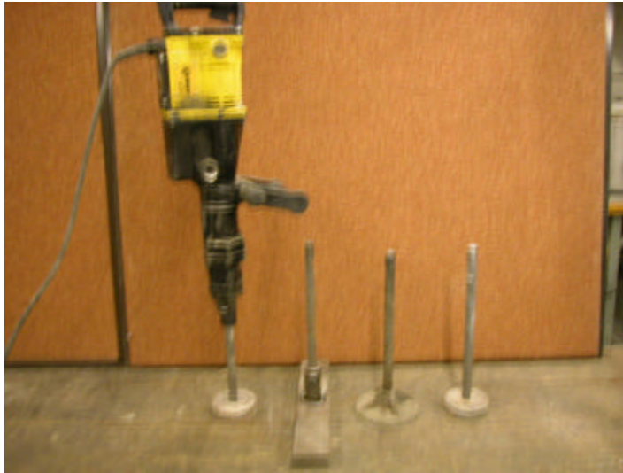
Fig. 1 – Vibratory Hammer and Tamping Plates for Cylinders and Beams
