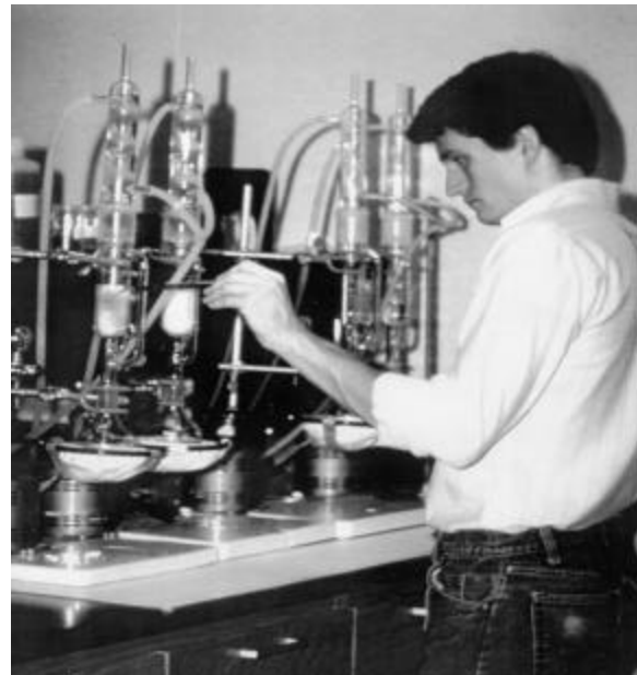
Figure 5.3. Soxhlet reactor (from Bradham and Caruccio, 1995)
