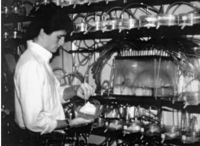
Figure 5.1. Humidity cells (from Bradham and Caruccio, 1995)
