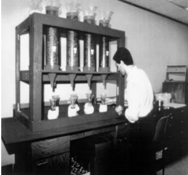
Figure 5.2. Leaching Columns (from Bradham and Caruccio, 1995)
