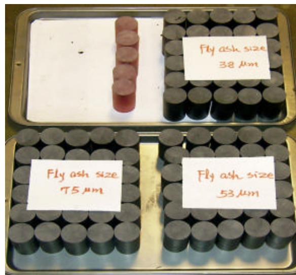
Figure 4.14 - Prepared ASTM samples for compression test
