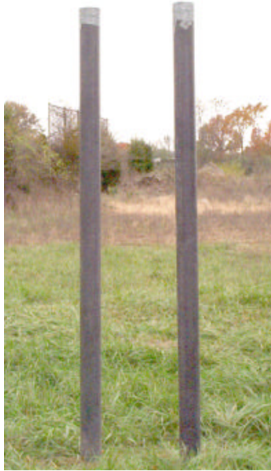
Figure 10.9 - Model composite poles installed outdoor at Illinois Coal Development Park (Fall 2002)
