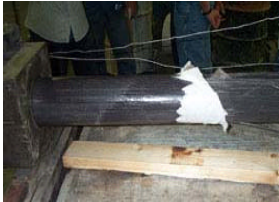
Figure 5.5 - Pultrusion of the model composite utility pole
