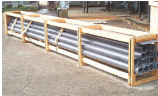
Figure 5.6 - Pultruded CCBs-filled FRC utility model poles
