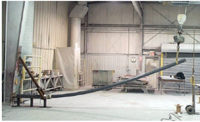
Figure 10.3 - Cantilever bending test of 20-ft long model composite utility pole
