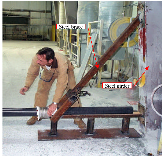
Figure 10.1 - The steel frame used to clamp the model pole
