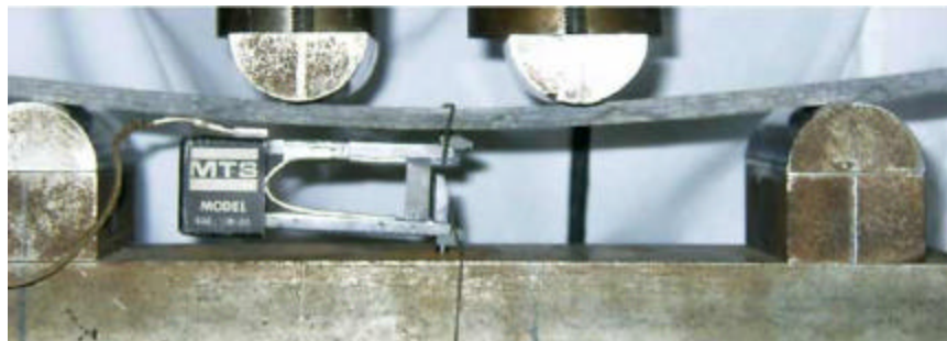
Figure 8.20 - Four-point flexural bending test of composite panel
