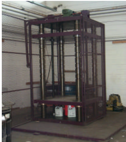
Figure 3.1- A 300,000 lb capacity compressive strength testing facility
